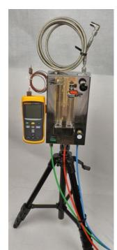
The temperature of the condensate is maintained above 80°C by controlling the steam flow through the inlet needle valve whilst measuring the temperature of the condensate via a thermocouple fitted to the outlet of the condenser.
