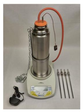
Whilst this method is not regarded as a truly accurate measurement of moisture in the steam, it can be used to demonstrate acceptable or otherwise dryness for sterilisation purposes. A dryness value of 1.0 is equivalent to 'dry saturated steam'. For sterilisation purposes a factor of 0.9 is acceptable for non-metal steriliser loads and for loads containing metal, a factor of 0.95.
