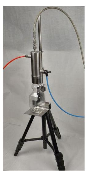
The 316 stainless steel, clean steam condenser is very efficient and compact and the condensate sample is collected cleanly due to the design shape of the condenser outlet. The condenser, pitot tube, isolating valve and steam supply tubing is required to be depyrogenated before use and this can be carried out in a suitably dry heat steriliser/oven at 180°C for three hours prior to their use.
